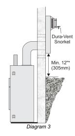
\*Diagam 3 & 4: As specified in CGA B149 Installation Code. Local codes or regulations may require different clearances.
